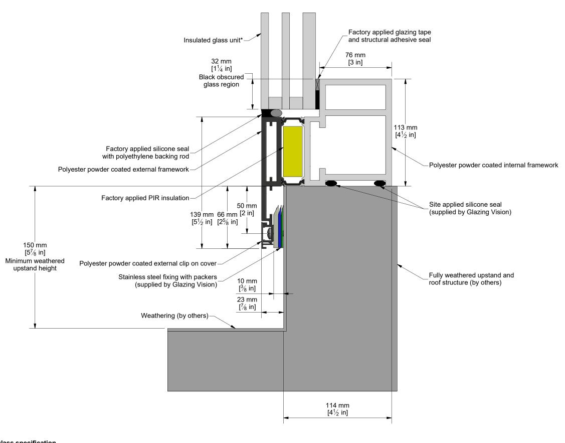
GLASS CONFORMS TO IMPACT RESISTANCE AND BREAKAGE CHARACTERISTICS OF BS EN 12600:2002. IGUS FABRICATED TO BS EN 1279 AND SUPPLIED IN ACCORDANCE WITH BS
