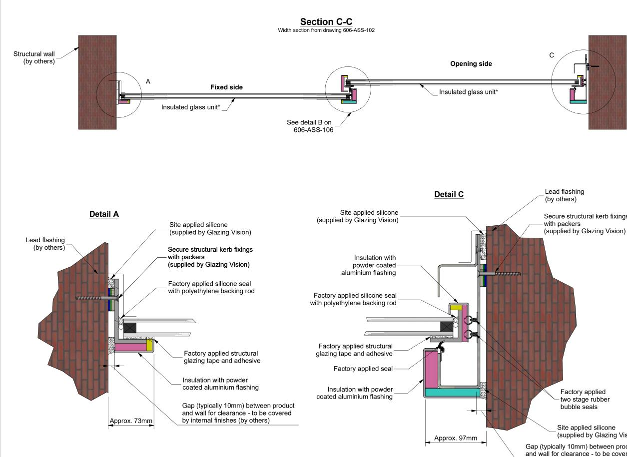
\*Example glass specification: 6mm clear toughened outer pane 16mm Black silicone sealed argon filled cavity with warm edge spacer 6mm clear toughened inner pane with soft low E coating
