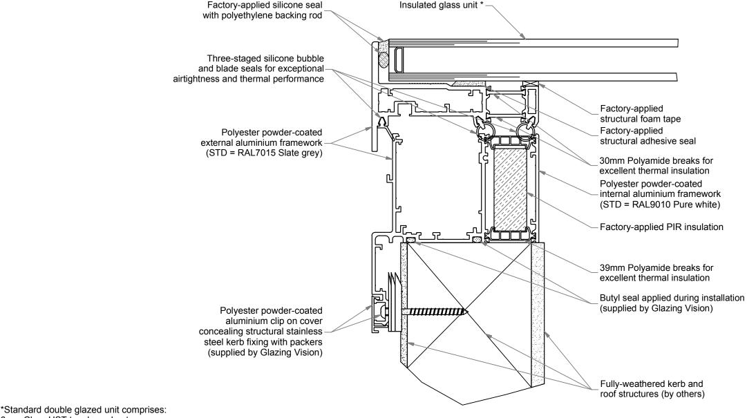
6mm Clear HST toughened outer 20mm Warm edge argon filled silicone sealed spacer 6mm Clear HST toughened soft coat low E inner
