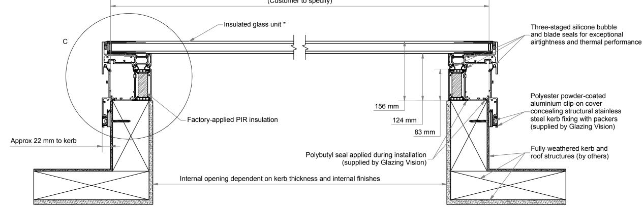
\*Standard double glazed unit comprises: 6mm Clear HST toughened outer 20mm Warm edge argon filled silicone sealed spacer 6mm Clear HST toughened soft coat low E inner
