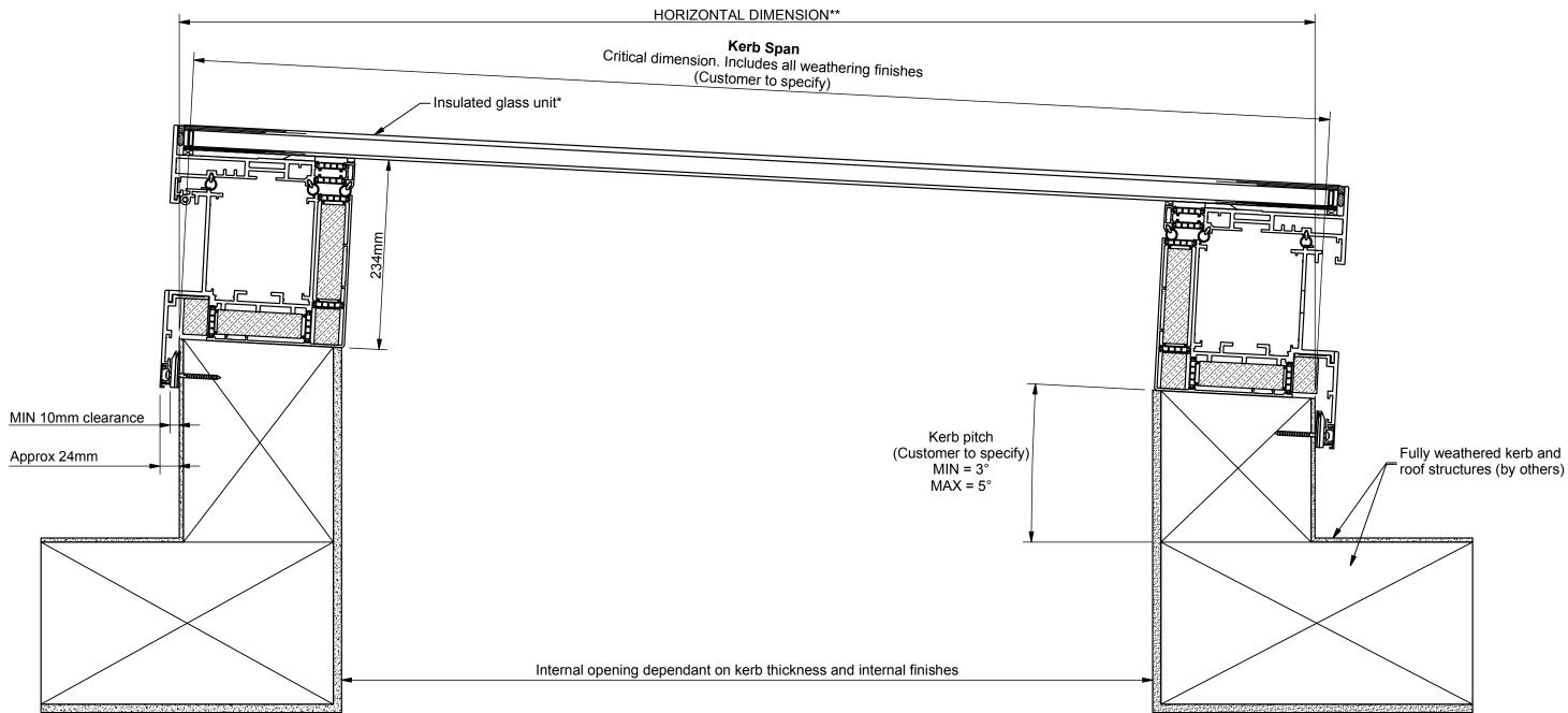
\*Standard double glazed unit comprises: 6mm Clear HST toughened outer 20mm Warm edge argon filled silicone sealed spacer 4mm Clear HST soft coat low E toughened inner
