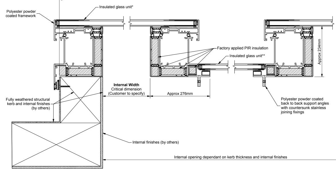
\*Standard double glazed unit comprises: 6mm Clear HST toughened outer 20mm Warm edge argon filled silicone sealed spacer 4mm Clear HST soft coat low E toughened inner \*\*Standard double glazed unit comprises:
