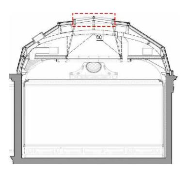
The architectural drawing above demonstrates how Glazing Vision's rooflight (highlighted in red) was installed within the apex section at the very top of the building.
