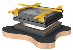
Figure 8 – Suggested lifting configuration
