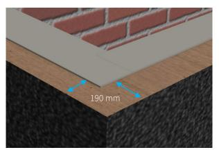
Figure 2 – Upstand top trim measurements
