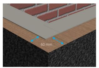
Figure 2 - Upstand top trim measurements
