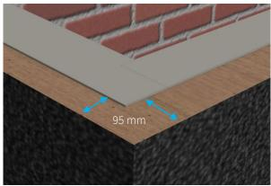
Figure 2 – Upstand top trim measurements
