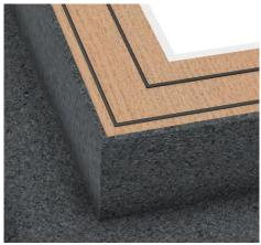
*Figure 5 – Silicone placement*
