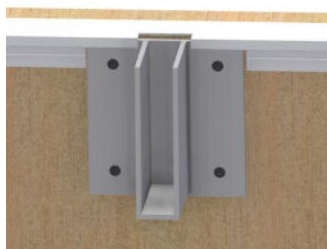
Figure 29 – Glass fin support bracket with upstand top trim
