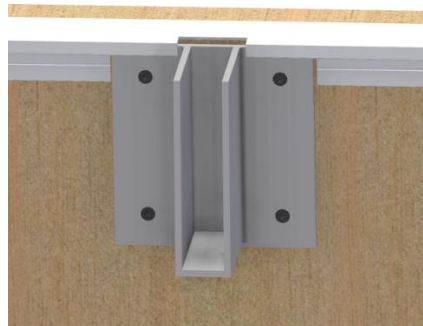
Figure 24 – Glass fin support bracket with upstand top trim
